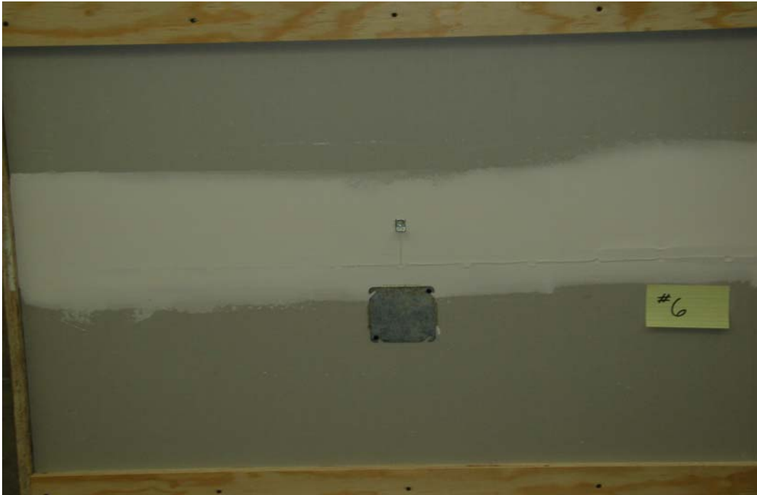
Figure 8 – Compression Failure – ButtTaper joint on 2x4 failure load = 8145 lbs
