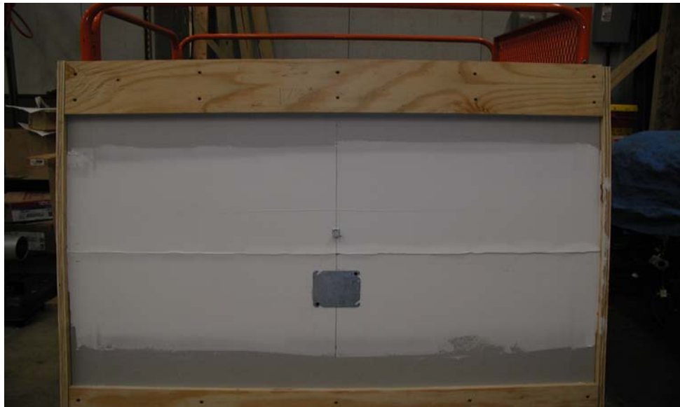
Figure 6 – Compression Failure – Standard joint on 2x4 failure load = 6627 lbs
