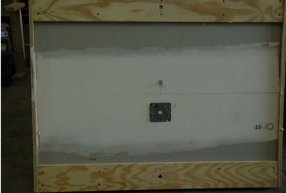
Figure 9 – Tension Failure – Standard joint on 2x4 failure load = 1547
